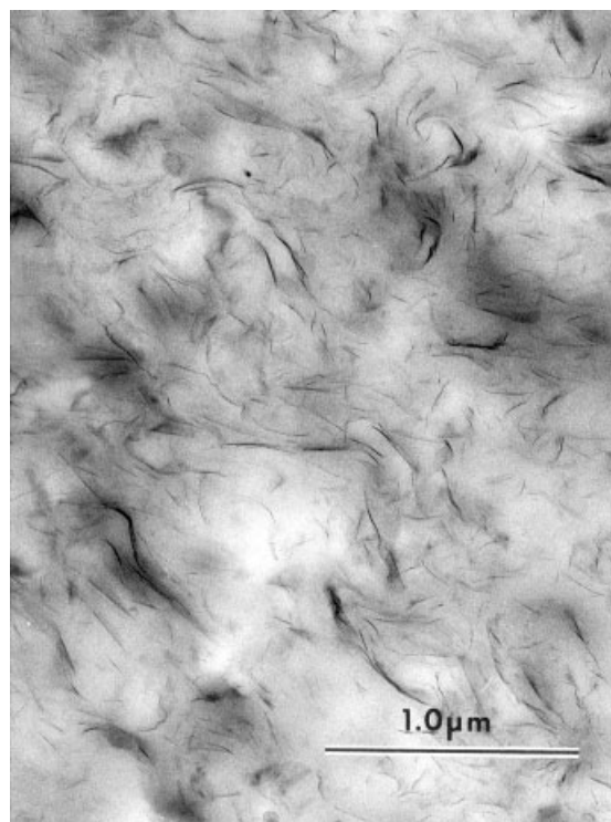
Figure 9 Low-magnification TEM image of a PPgMA intercalated/exfoliated nanocomposite (mass fraction = 8% A-MMT).
