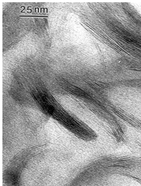
Figure 4 High-magnification TEM image of a novalac-based cyanate ester nanocomposite (mass fraction = 10% MEL-MMT) that gave no peak by solid-sample XRD but did when the sample was powdered.
