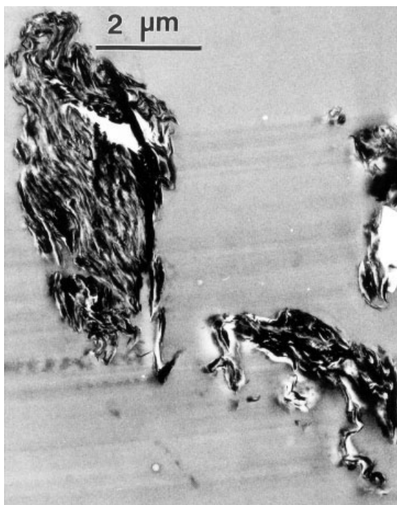
Figure 2 Low-magnification TEM image of an immiscible novalac-based cyanate ester nanocomposite (mass fraction = 10% MEL-MMT) that gave no peak by XRD.
