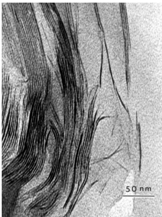
Figure 8 High-magnification TEM image of an intercalated/exfoliated PS nanocomposite (mass fraction = 5% A-MMT). This is a different region of the same sample shown in Figure 6, illustrating a large intercalated region.
